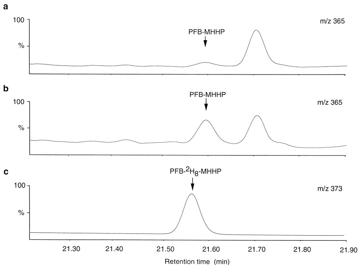
Fig. 4. Chromatograms of the fragment  $m/z$  365 for MHHP acid of (a) a sample from a non-exposed subject, (b) a single human sample containing 0.9 pmol HHP acid and (c) the fragment  $m/z$  373 from the deuterium-labeled internal standard.
