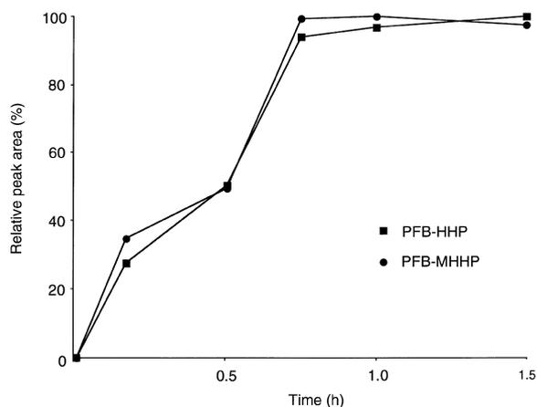
Fig. 2. The relative peak areas for di-pentafluorobenzyl hexahydrophthalate and di-pentafluorobenzyl methylhexahydrophthalate after various times of derivatisation. Each mark denotes one single determination.
